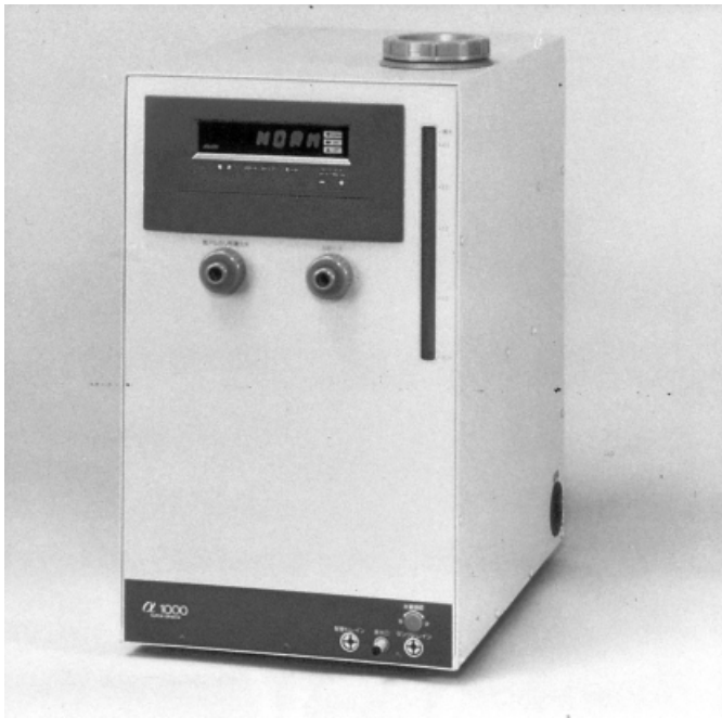
Fig. 1. Strongly acidic electrolyzed water generator used for this experiment: \alpha 1000 320 (w) \times 460 (d) \times 570 (h); produces 1000 mL/min of SAEW; storage tank is necessary.
