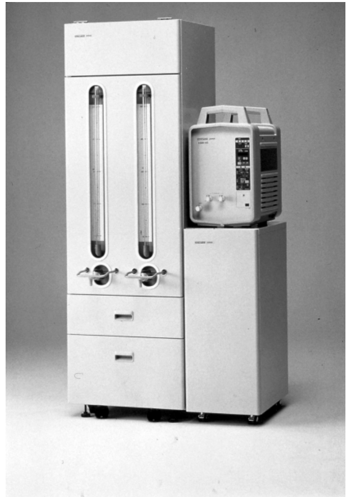
Fig. 2. Strongly acidic electrolyzed water generator used in this experiment: overview of ESW-45 with storage tank; generator: 290 (w) \times 510 (d) \times 510 (d); 750 mL/min of SAEW from tap water; tank stores 100 L max. of SAEW.
